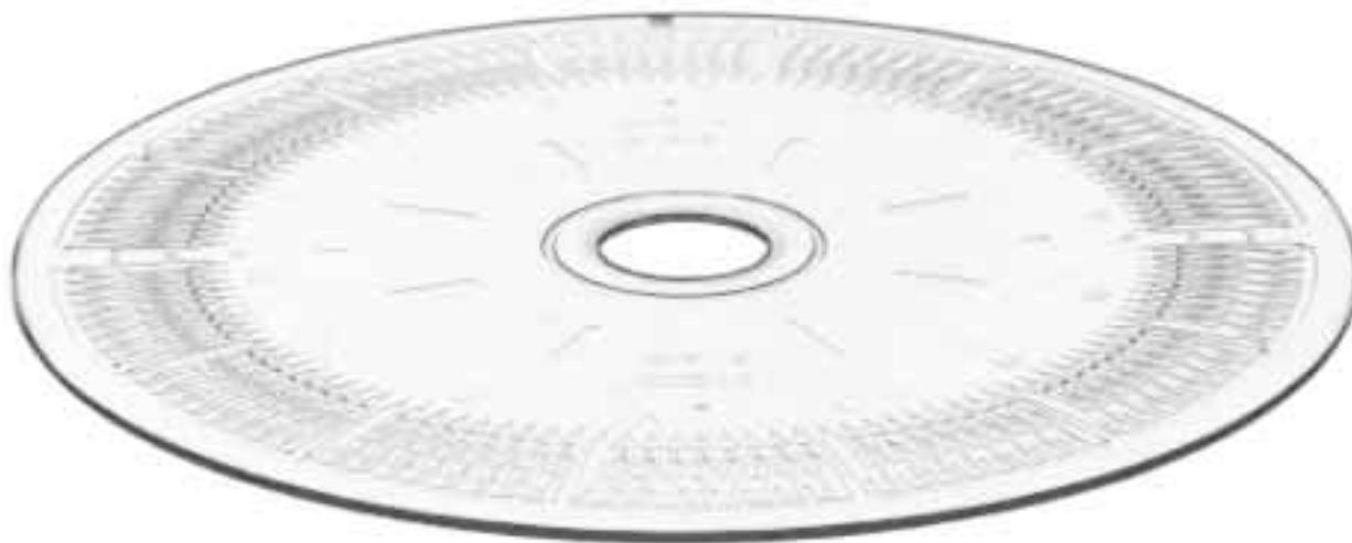
**Figure 4.** Photograph of the Lab-on-a-Disc. The 104 structures incorporated into a single CD (12 cm in diameter). Reprinted with permission from Ref[12].
