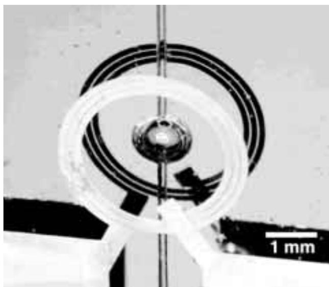
**Figure 12.** Scanning electron micrograph of a microfabricated Helmholtz coil. Fluidic microchannels are seen on top and bottom to interface spherical sample chamber with the external world. Reprinted with permission from Ref[35].
