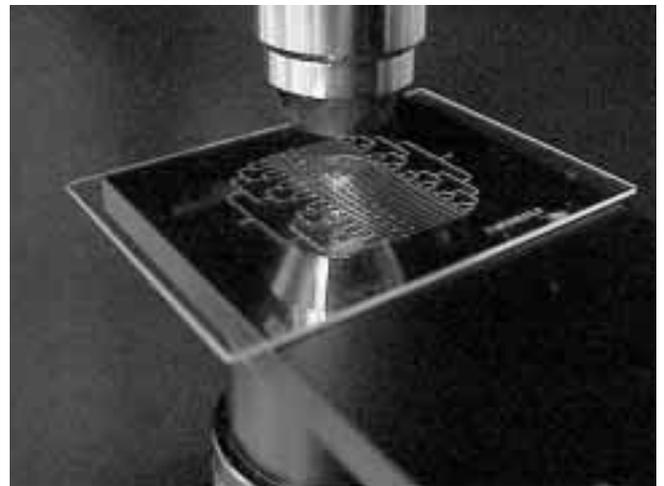
**Figure 9.** Photograph of a thermal lens microscope (Institute of Microchemical Technology Co., Ltd. with permission).
