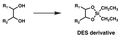
Figure 5. Derivatization of hydroxyl groups with N, O-bis (diethylhydrogensilyl) trifluoroacetamide.
