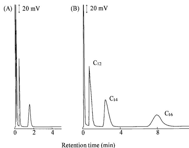
**Figure 14.** Comparison of fiber-packed column (A) and coated-fiber-packed column (B). For the fiber coating, HR-1701 (Shinwa Chemical, Kyoto, Japan) was used. Other conditions were the same as in Figure 12, except for the column length of 1 m and the temperature at 80 (isothermal).
