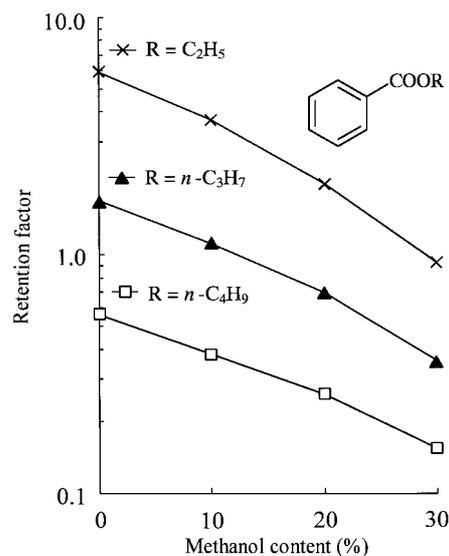
**Figure 10.** Effect of methanol content in the mobile phase on the retention on alkyl benzoates. Conditions : column, fused-silica (0.20 mm i.d. × 50 mm ; total length 500 mm) packed with Zylon<sup>®</sup> (HM) fibers, mobile phase, methanol/Tris-HCl buffer (2.5 mM, pH = 8.6). Other conditions are the same as in Figure 9.
