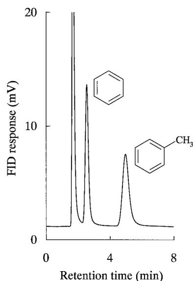
**Figure 12.** Typical GC separation of benzene (a) and toluene (b) with Zylon<sup>®</sup> (HM) fiber-packed column. Conditions : column size, 0.32 mm i.d.  $\times$  2 m ; column head pressure, 100 kPa ; column temperature, 50 ; injector and detector temperature, 250 ; split ratio, (50 : 1).
