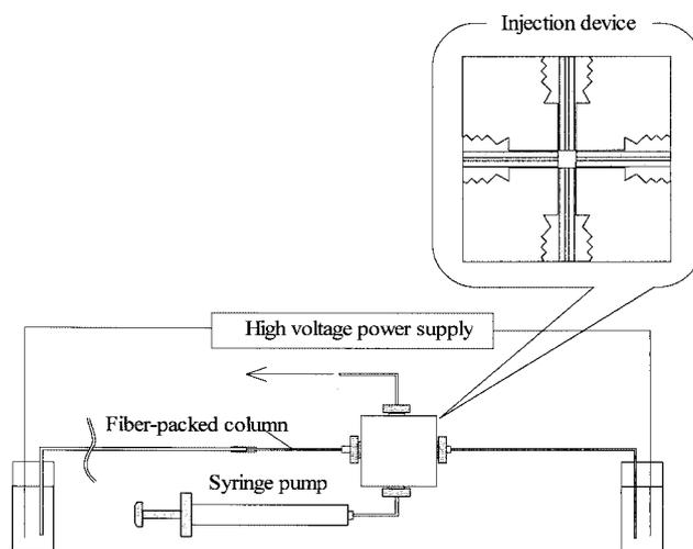
**Figure 8.** Overview of the fiber-packed CEC system.
