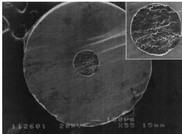
**Figure 2.** SEM images of typical "fiber-in-tube".
