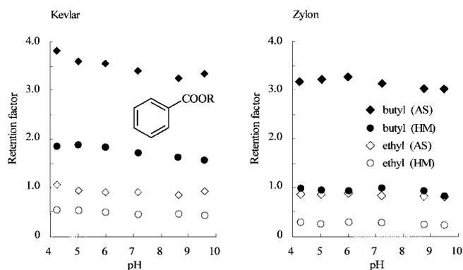
**Figure 11.** Effect of pH on the retention of *n*-alkyl benzoates. Conditions : column, fused-silica (0.20 mm i.d.  $\times$  50 mm ; total length 700 mm) packed with different fibers. Mobile phase was prepared with various buffer solutions having different pH values.
