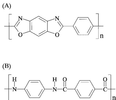
**Figure 1.** Chemical structures of Zylon<sup>®</sup> (A) and Kevlar<sup>®</sup> (B).
