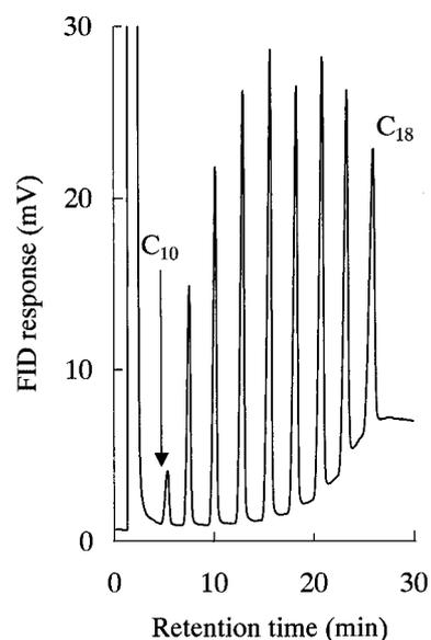
**Figure 13.** Typical chromatograms for the separation of *n*-alkanes (C<sub>10</sub>-C<sub>18</sub>) mixture with Zylon<sup>®</sup> (HM) packed column. Conditions : column size, 0.32 mm i.d.  $\times$  2 m ; column temperature, 80 to 200 at 5 /min ; split ratio, (50 : 1) ; column head pressure, 200 kPa ; injector and detector temperature, 300 .
