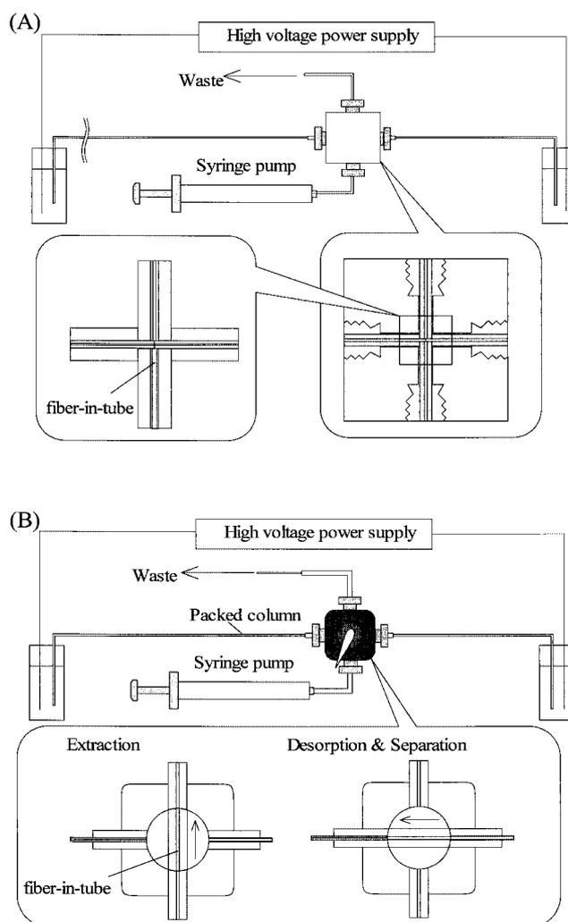
**Figure 5.** Schematic diagram of fiber-in-tube SPME/CE (A) and fiber-in-tube SPME/CEC (B) system.
