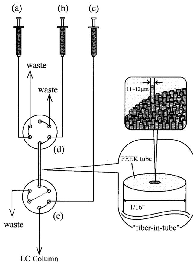
**Figure 3.** Schematic diagram of fiber-in-tube SPME/micro-LC. Syringe pumps for sample solution (a), desorption solvent (b) and mobile phase (c), and switching (d) and injection (e) valves.
