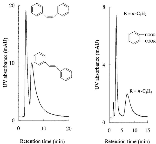
**Figure 7.** Typical chromatograms for the separation of cis-/trans-stilbene mixture (A) and di-*n*-alkyl phthalates (B) with fiber-packed column in LC. Conditions : mobile phase, methanol/water = 50/50 (A), 30/70 (B) at the flow-rate of 20  $\mu$ L/min ; injection volume 1  $\mu$ L ; detection, UV at 254 nm.
