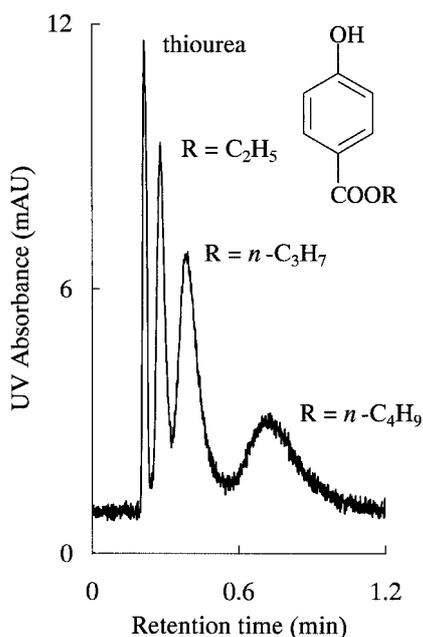
**Figure 9.** Chromatogram for the separation of *p*-hydroxy-*n*-alkyl benzoates with fiber-packed column. CEC conditions : column, fused-silica (0.20 mm i.d. × 50 mm ; total length 700 mm) packed with Kevlar<sup>®</sup> (AS) fibers ; mobile phase, 2.5 mM sodium phosphate buffer (pH = 7.0) ; injection 5 kV (5 sec) ; applied voltage, 20 kV ; detection, UV at 254 nm.
